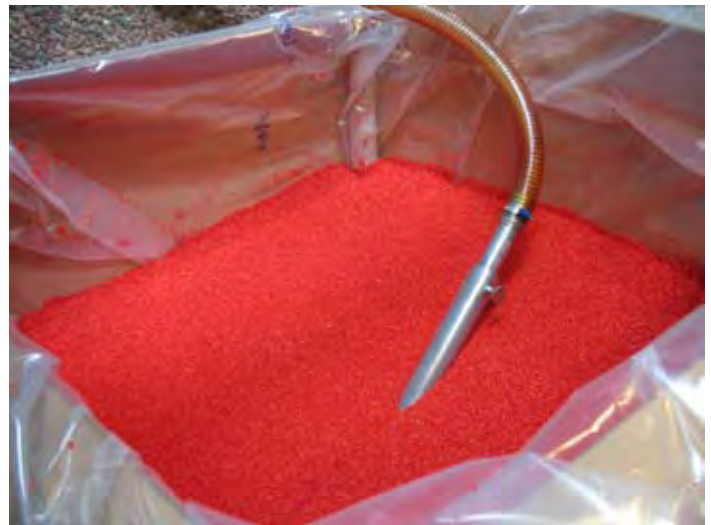
Plastic granules - the raw materials used for making LEGO elements
