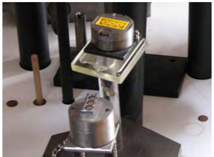
The two halves of a mold. Plastic is injected into the mold to make the 2 x 4 brick shown.
